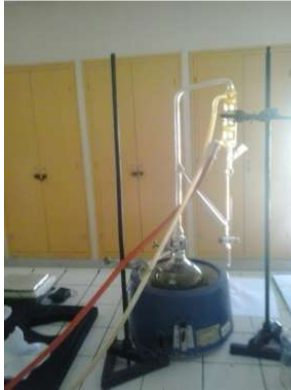
Figure 1. Special laboratory hydro-distillation apparatus (Clavenger). Source: Elkacimi (2016).
