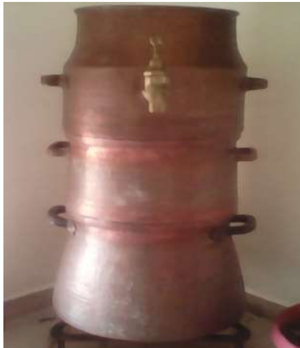
Figure 2. The artisanal alembic - type "Alquitara" used in this study. Source: Elkacimi (2016).
